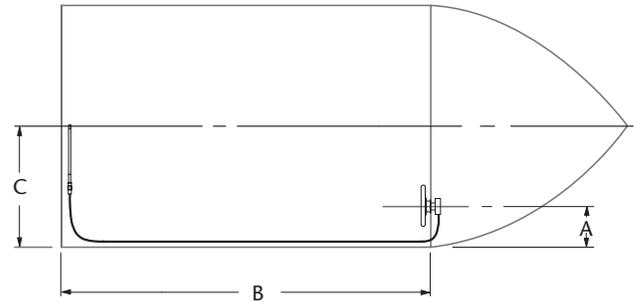
A single-cable, starboard drive push-pull mechanical cable system is shown in this diagram. If your mechanical system is different than the one depicted and/or you have any questions about mechanical steering after reviewing this guide, please contact Teleflex Technical Service.
